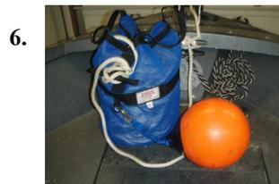
Attach a small buoy to the D-ring below the cleat. This will mark your bag and reduce the chance of running over it.
