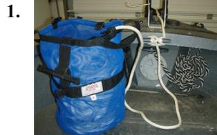
Anchor has been deployed. Line is tied off to the cleat at bow.
